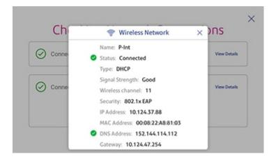
If for any reason your meter cannot connect to the network, the validation process stops here. In this case, tapping **View Details** will show the status of the wireless settings like the one shown in the example below.
