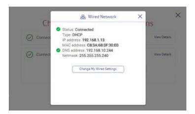
If for any reason your meter cannot connect to the network, the validation process stops here. In this case, tapping **View Details** will show the status of the wired settings like the one shown in the example below.
