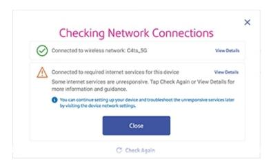
To identify the specific services that the tool cannot connect to, tap **View Details**. An example of the View Detail screen is shown here.
