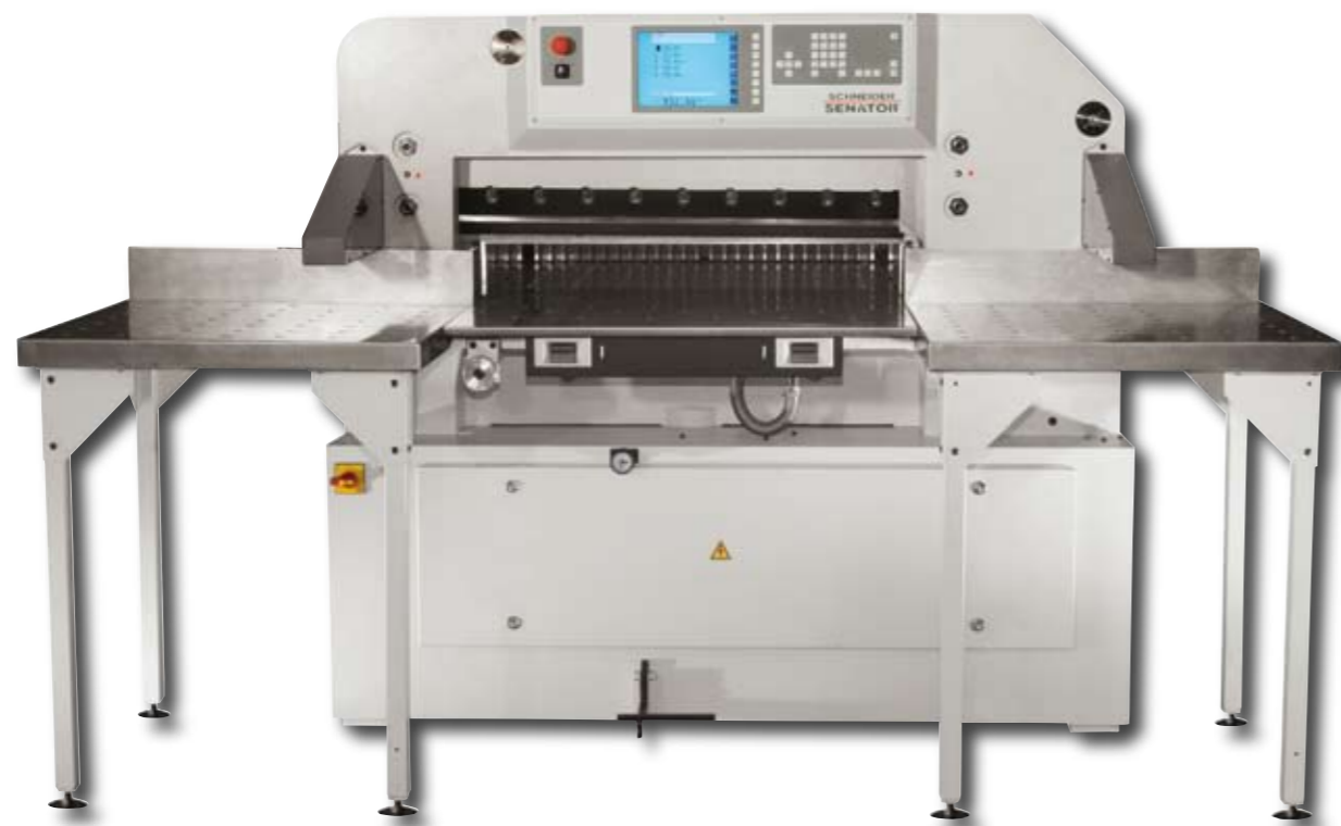
The illustration shows the machine including airfilm side-tables LST 750 with stainless steel surface, rustproof.
