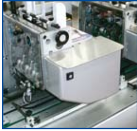
Rotary insert feeder featuring suction cups, single gripper and rotary drum.
