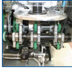
Disk attachment for processing open edge inserts on the rotary feeders.
