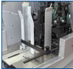
The shuttle feeder can be interchanged with the rotary feeders and allows for the feeding of catalogues and CDs.
